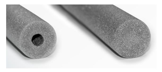
NOMATEC® Backer Rod Hollow & Full round profiles are manufactured from closed-cell polyethylene foam and are used as backing material for elastomeric and other cold-applied sealants. They are inserted into a joint to control the sealant depth and act as bond-breakers, without adhering to the sealant.
