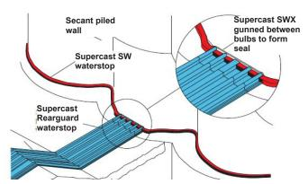
Supercast SW, Supercast SWX and Supercast Rearguard waterstops at secant pile wall and floor slab junction
