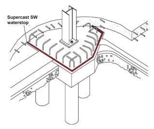
Pile cap detail using Supercast SW waterstop
