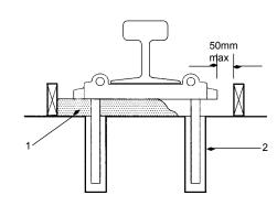
Example of Conbextra EP grout to machinery baseplate:
