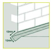
Form chase at wall to floor and all internal wall angles minimum IOmm x IOmm.
