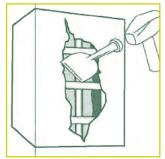
Cut back loose and spalling concrete a minimum depth of 10mm.
