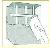
Mix NATCEM 35 as instructed and place the mortar, ensuring at all times a minimum thickness of 10mm.
